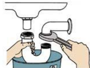
Cover the chrome nuts with tape to prevent marring.
