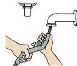
Loosen the thumb screw and move the handle about 3' from the end of the snake.
